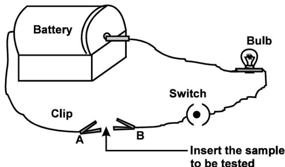
**Step 2:** Place the metal to be tested in the circuit between terminals A and B.
