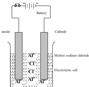
**Reaction at Cathode:** The positively charged aluminium ions ( $\text{Al}^{3+}$ ) are moved towards the cathode and they takes electrons from the cathode and get reduced to form aluminium atoms.
