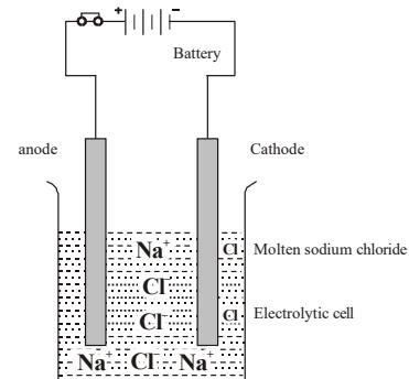
During the electrolysis of molten sodium chloride the following chemical reactions take place at cathode and anode.
