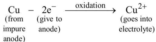
As the process goes on, impure anode rod becomes thinner and thinner. Whereas pure cathode rod becomes thicker and thicker in this way pure copper is obtained at the cathode and impurities like gold and silver present in the impure copper rod are collected below the anode which is called **anode mud**. Thus, the electrolytic refining of metals serves two purposes these are:
